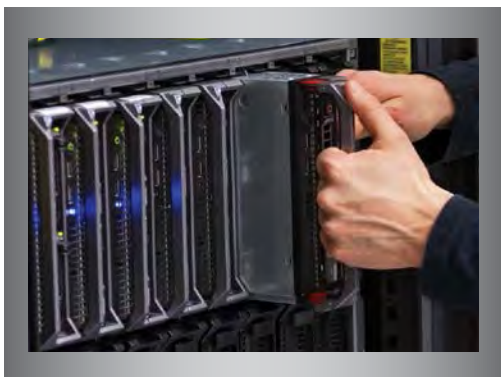
Blade servers and other high-density, high-wattage loads can create problematic hot spots if they're installed too close to each other.
